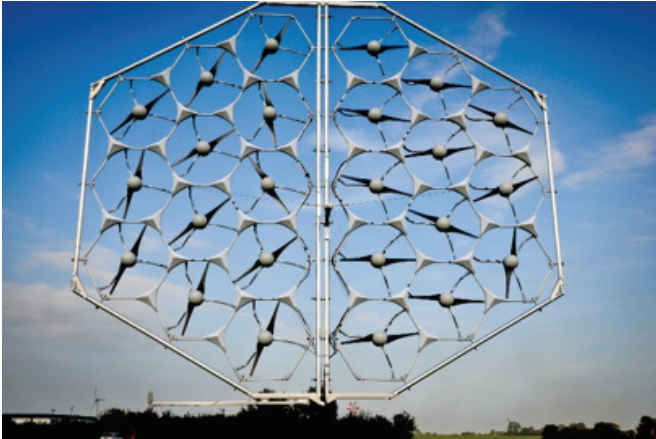
Fig. 1: Free-field test of a 10-kilowatt modular turbine system in northern Germany. Official measurement by Germanischer Lloyd
